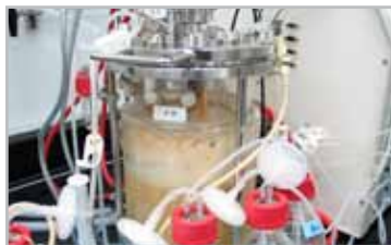
Foaming at high sparge rate in conventional bioreactor
